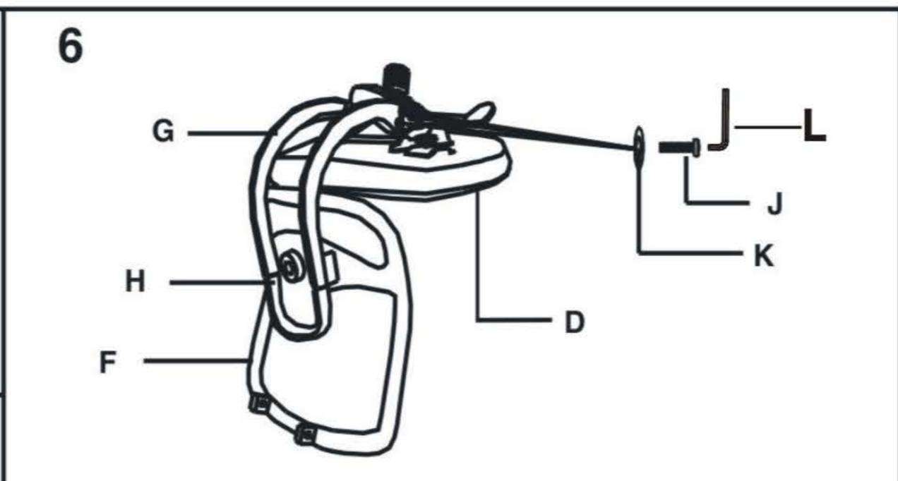
according to the picture, use screws to connect mechanism and back frame.
