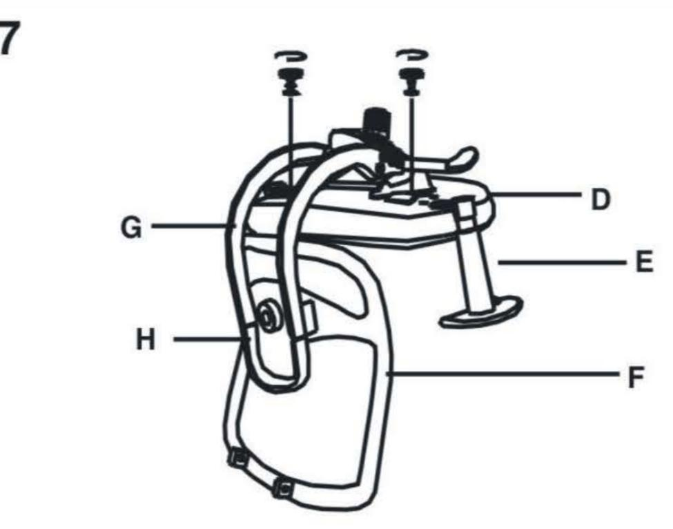
Loose out two wheels from the steel sheets, then insert "E" under the steel sheets, tighten the wheel.
