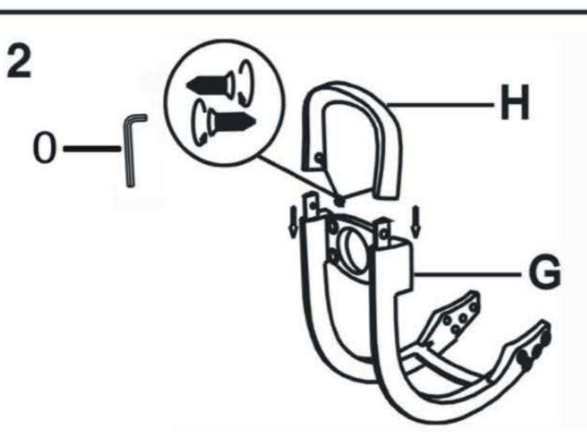
insert"H"part into"G"then assemble two screws back and tweak tightly.
