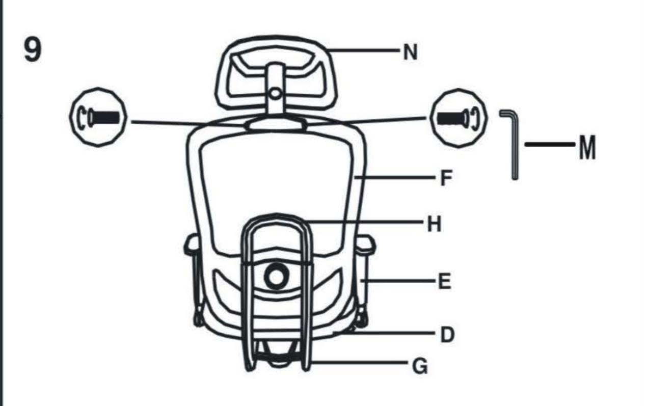
Put"N"to"F"at the right position then tighten the two screws.
